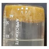
Sand Consolidation, SandLink two part system at 10 L/ton frac sand:
