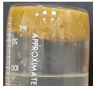
*Sand Consolidation, SandLink two part system at 10 L/ton frac sand:*
