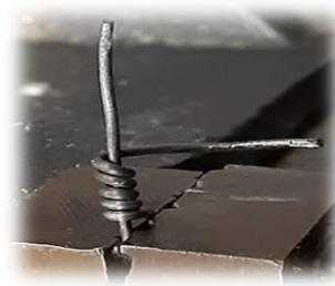
**WL-HCL-28 (Diluted 1:2 v/v with water), 90C for 12 hrs Exposure**
